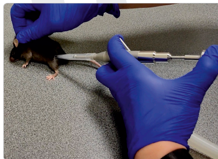
A single person can perform the collection process from mice. The vacuum sucks the hairs between the forceps squeezed by the thumb operated piston.
